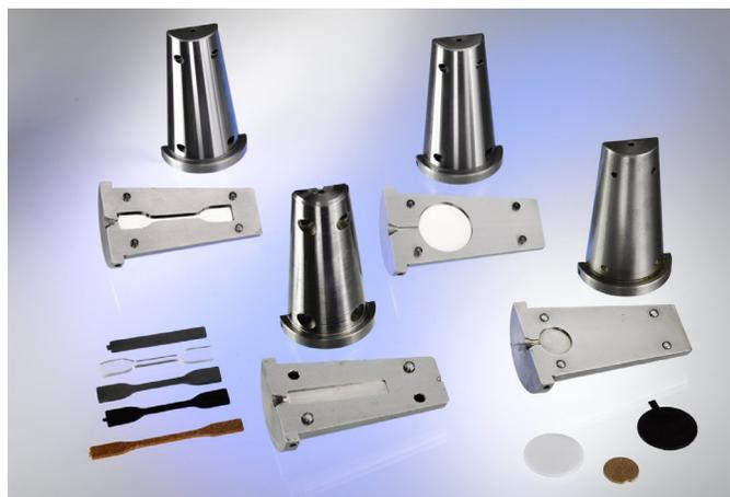
Figure 6: HAAKE MiniJet molds with injection molded samples of different shape and size.
