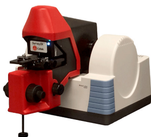
Figure 4. Nicolet iS5 FTIR spectrometer with the SurveyIR® Accessory in the sample compartment.
