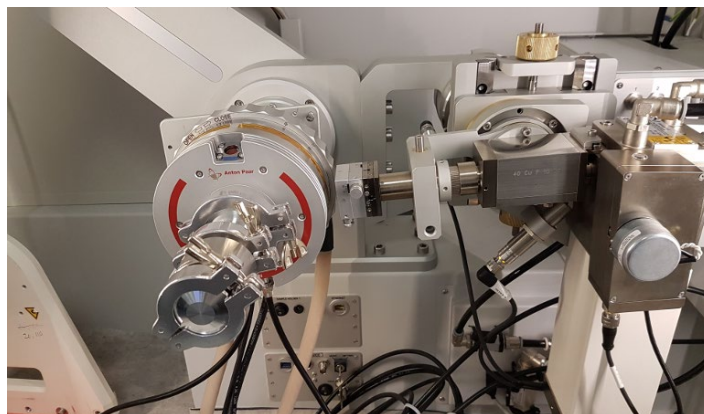
Figure 2: HTK16 installed on ARL EQUINOX 3500 instrument
