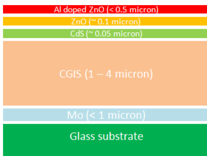
Figure 1: Cross sectional schematic of a typical CIGS solar cell.
