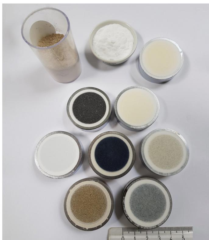
Figure 1. Pressed mineral sample pellets prepared for XRF analysis.
