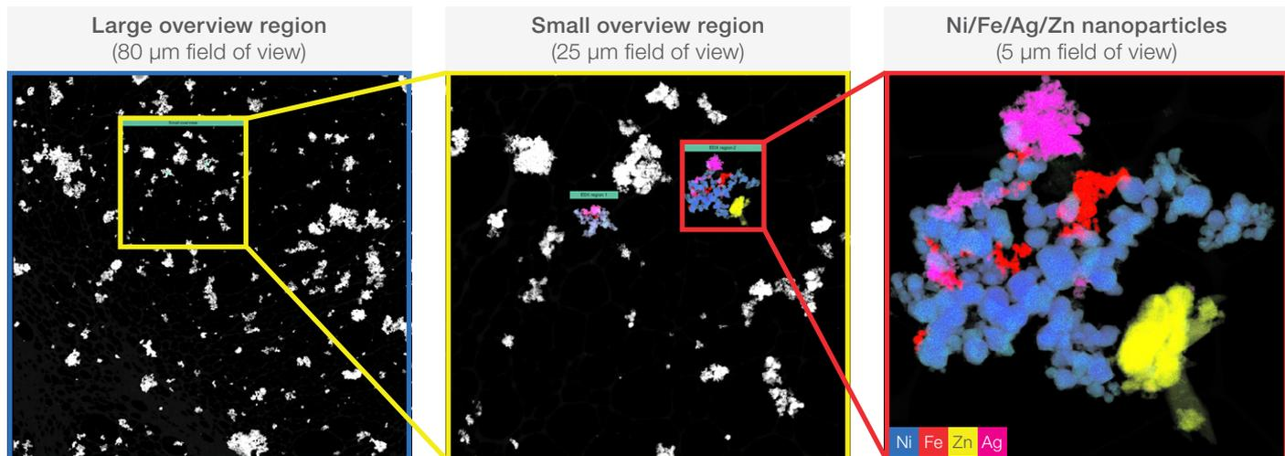
Figure 2. APW used on mixed nickel, iron, silver, and zinc catalyst nanoparticles. Different colors are assigned to represent different elements. This image was obtained in STEM mode with chemical information determined by EDS.
