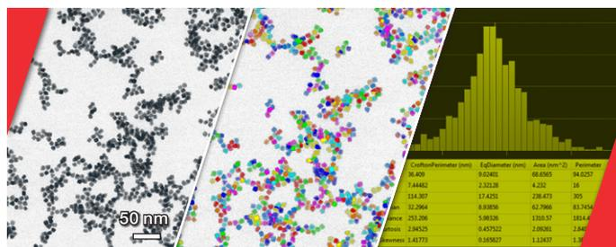
Figure 1. Automated, large-area TEM acquisition using APW for the analysis of individual nanoparticle parameters. *Sample courtesy of Prof. B. Gorman and Prof. R. Richards, Colorado School of Mines.*
