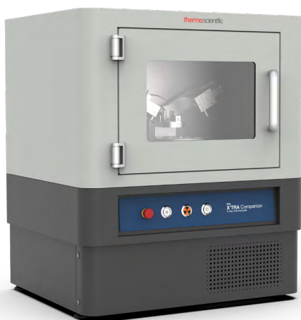
Figure 1. ARL X'TRA Companion diffraction system
