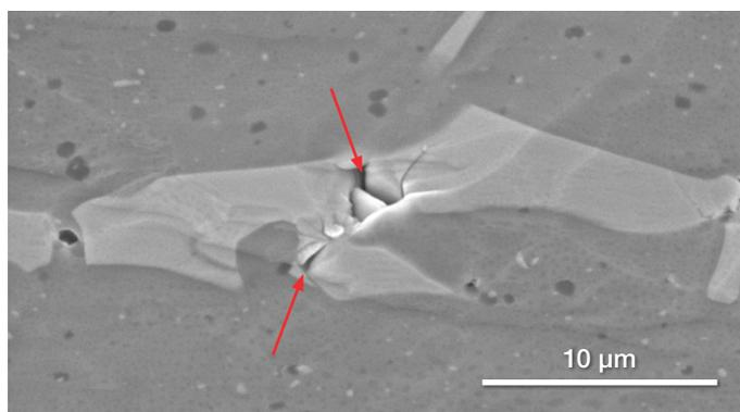
**Figure 2.** SEM image of an aluminum matrix. Arrows indicate microcracks associated with the bright Fe-rich particles. Dark Mg-Si intermetallic particles are also visible. *Sample courtesy of the University of Science and Technology Beijing.*
