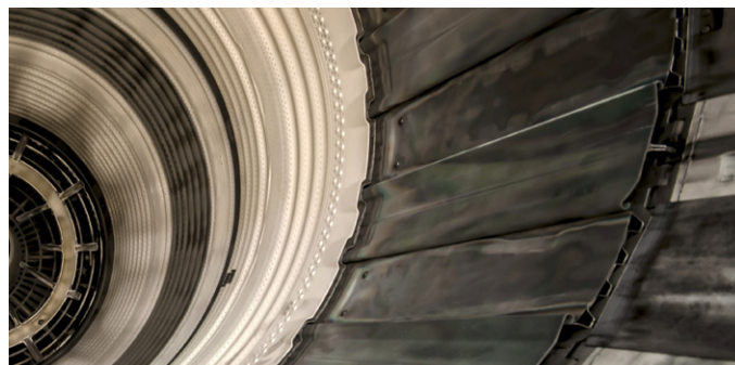
Figure 2. Rear view of an afterburner.
