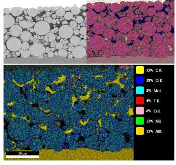
Thermo Scientific™ Avizo™ Software allows users to take advantage of the high-resolution grayscale image and the chemical low-resolution EDS image to produce advanced measurement on the granular structure in an easy and reproducible way.
