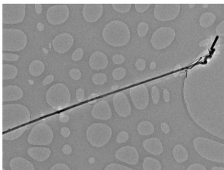
Figure 1a. Low magnification TEM image showing a geometry of B-Ni composite nanowire
