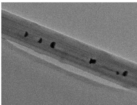
Figure 1b. TEM image showing the presence of Ni catalyst particles/fragments in Boron matrix
