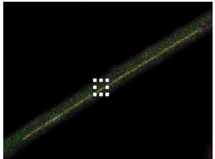
Figure 7a. DF-STEM image of B-Ni composite nanowire
