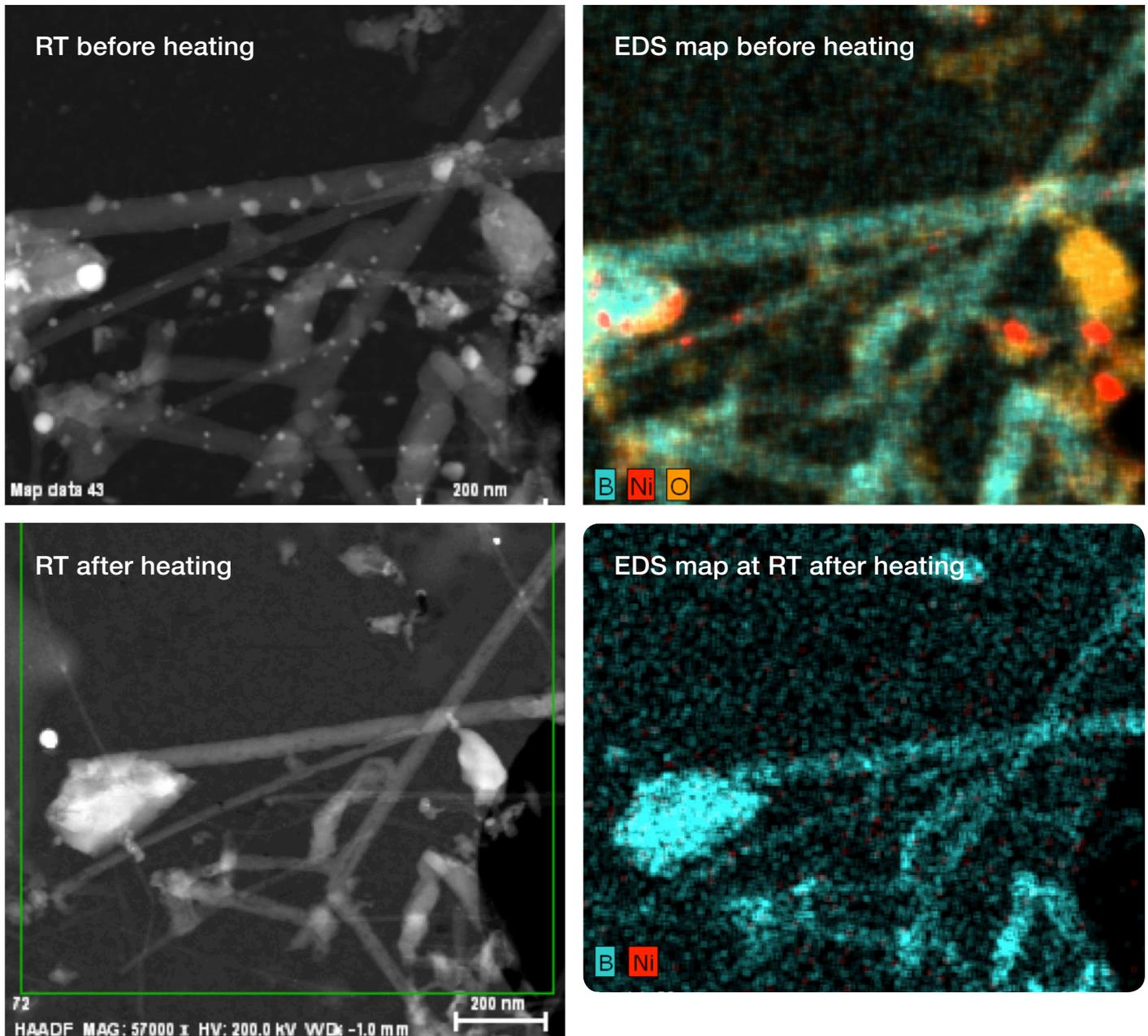
Figure 6. Corresponding EDS maps acquired at RT after cooling sample from 1200°C
