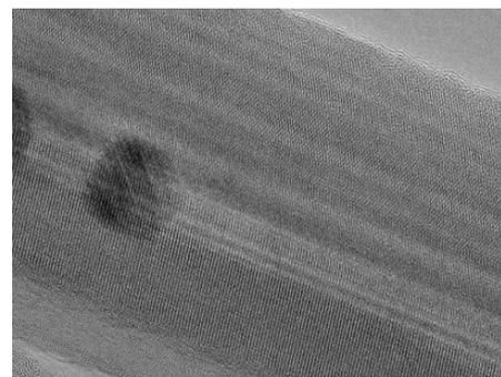
Figure 1c. HR-TEM image showing crystalline lattice of B shell and Ni nanocrystal
