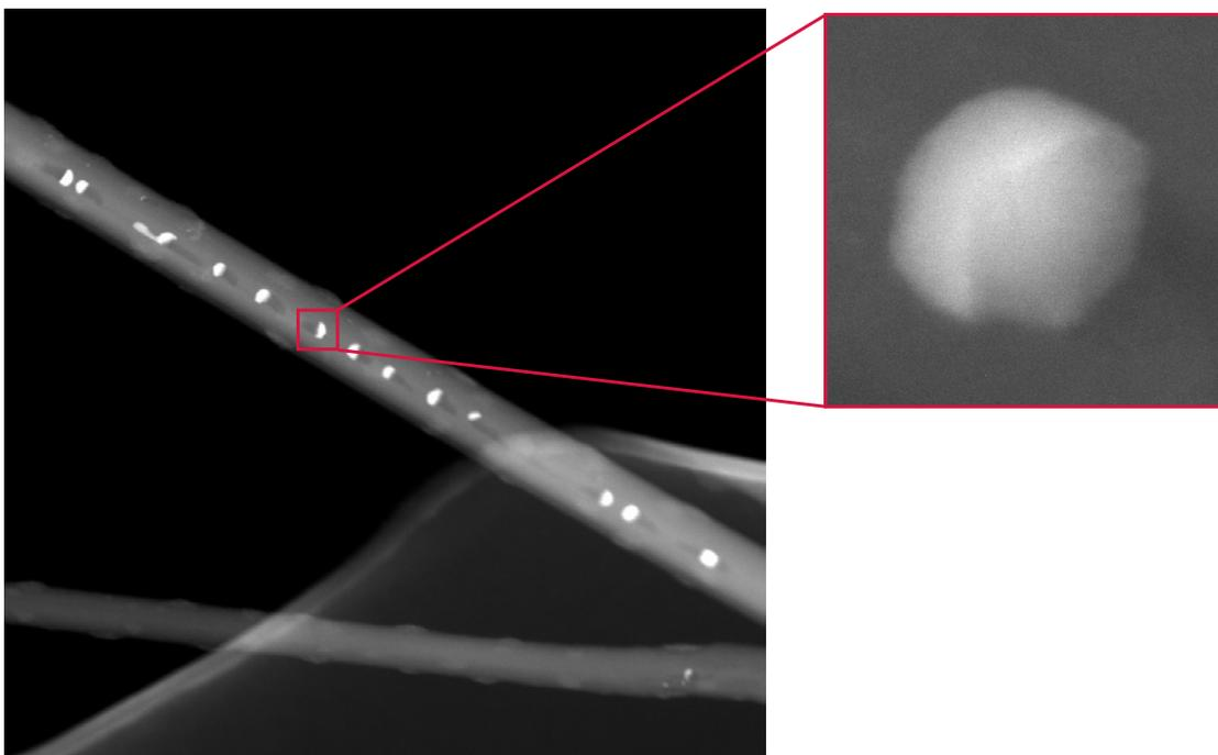
Figure 2. DF-STEM image revealing high contrast crystalline Ni fragments in Boron nanowire; Enlargement shows individual Ni crystal at higher magnification
