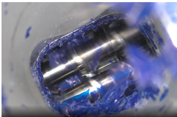
Figure 2: Large primary feed port of Thermo Scientific Process 16 twin-screw extruder with wide throat feed screw elements ensures uptake of larger foil shreds.
