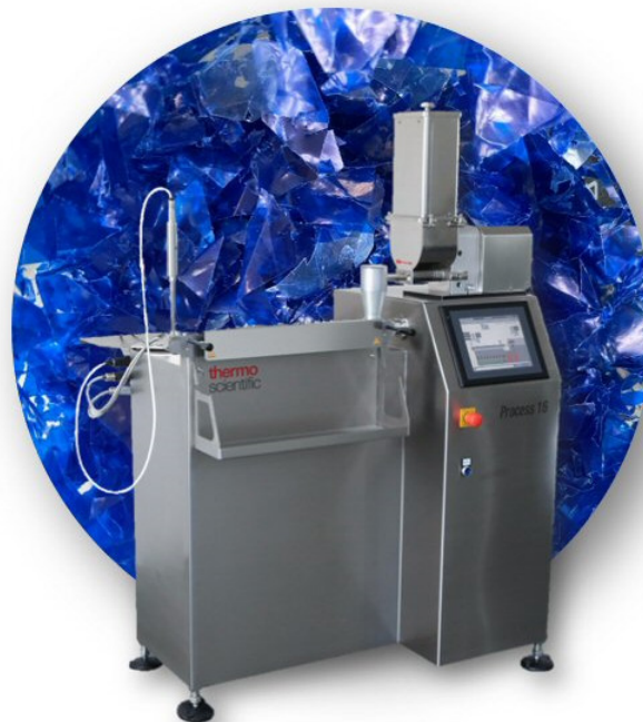
Figure 1: Thermo Scientific Process 16 twin-screw compounder and twin-screw feeder for foil shred recycling.
