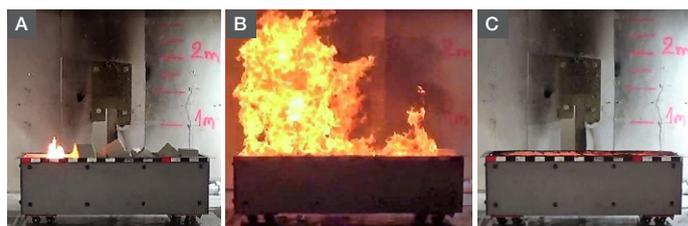
Figure 2. Photos of the foam tray a) at the beginning of ignition (t = 0), b) at t = 3 min, and c) at t = 5 min.
