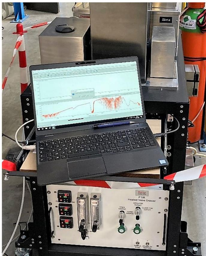
Figure 1. Photo of the Thermo Scientific Modular Gas Sampling System.
