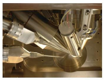
Figure 4: The inside of a DualBeam chamber
