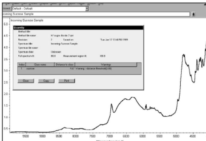
Figure 7. Spectrum of a sucrose sample contaminated with glucose.
