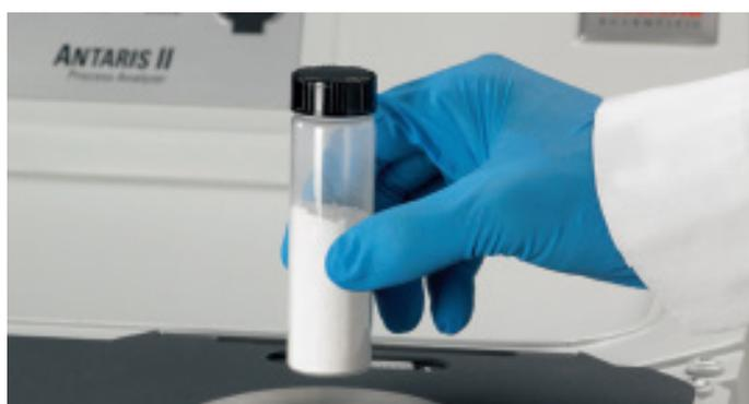
Figure 1. Powder analysis with the Antaris FT-NIR Analyzer.
