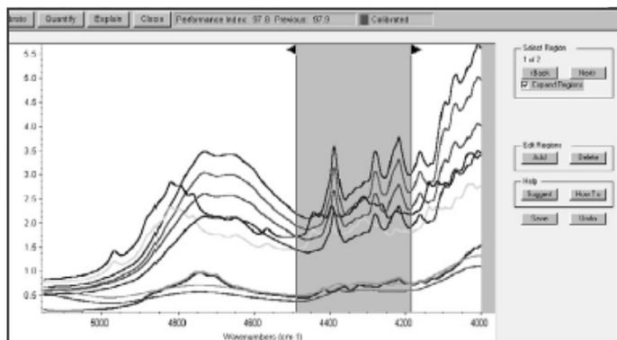
Figure 3. One of two spectral regions used to develop the classification model.
