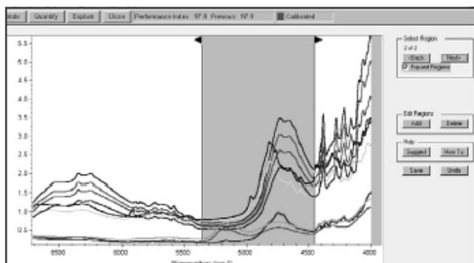
Figure 4. One of two spectral regions used to develop the classification model.
