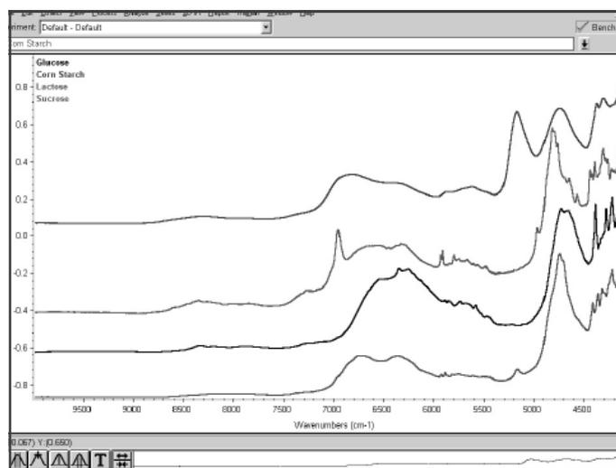
Figure 2. Example spectra of polysaccharide samples collected with the Integration Sphere Module on the Antaris FT-NIR Analyzer.
