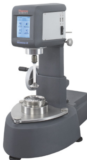
Figure 3: HAAKE Viscotester iQ Air with Peltier temperature control.
