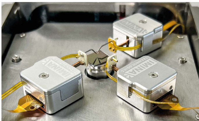
Figure 2. Imina Technologies miBot Probers placed around the Phenom sample holder.
