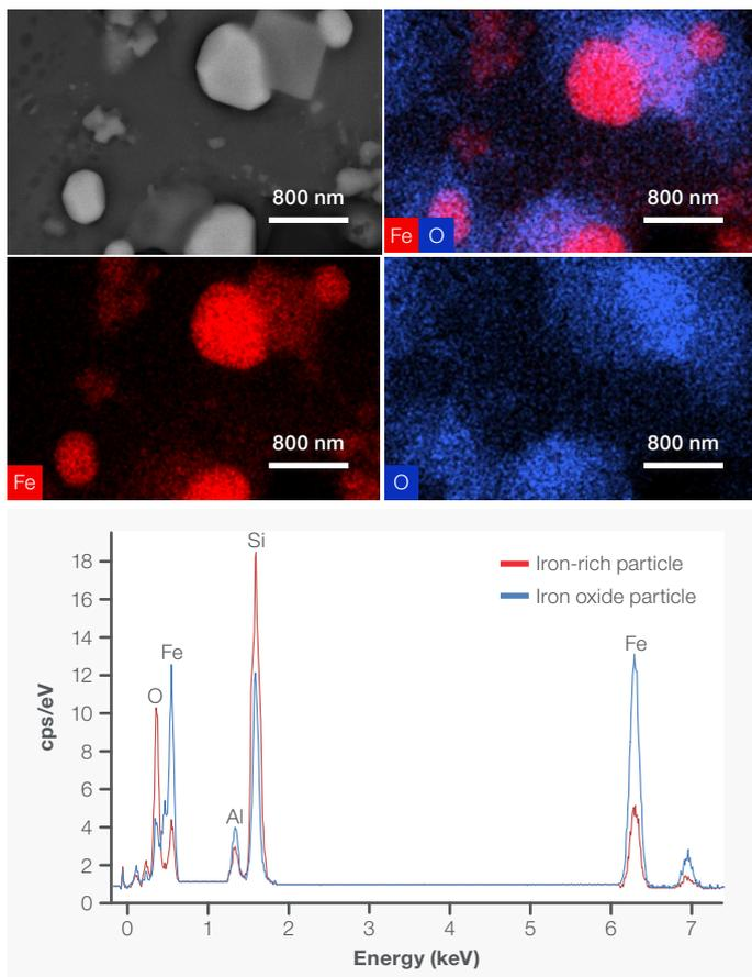
Figure 4. EDS mapping acquired on the heated area. The iron and oxygen maps show an inhomogeneous distribution of the iron in the three particles on the top right area of the image. The two spectra come from two particles showing different compositions.
