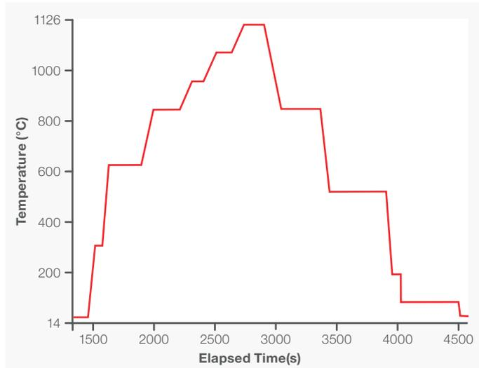
Figure 2. Temperature change in time. The first half of the graph shows the heating, in steps, up to 1,100°C. The second half shows fewer steps during cooling, as it was performed more quickly than the heating.
