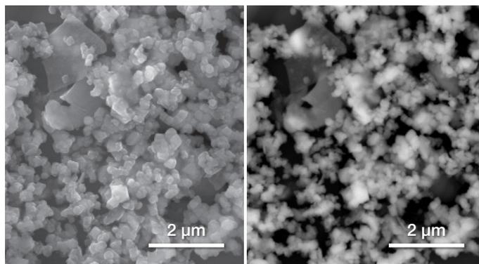
Figure 1. SE and BSE images acquired at the beginning of the experiment, with the temperature set at 40°C. Acc voltage 20 keV, beam current 0.13 nA.
