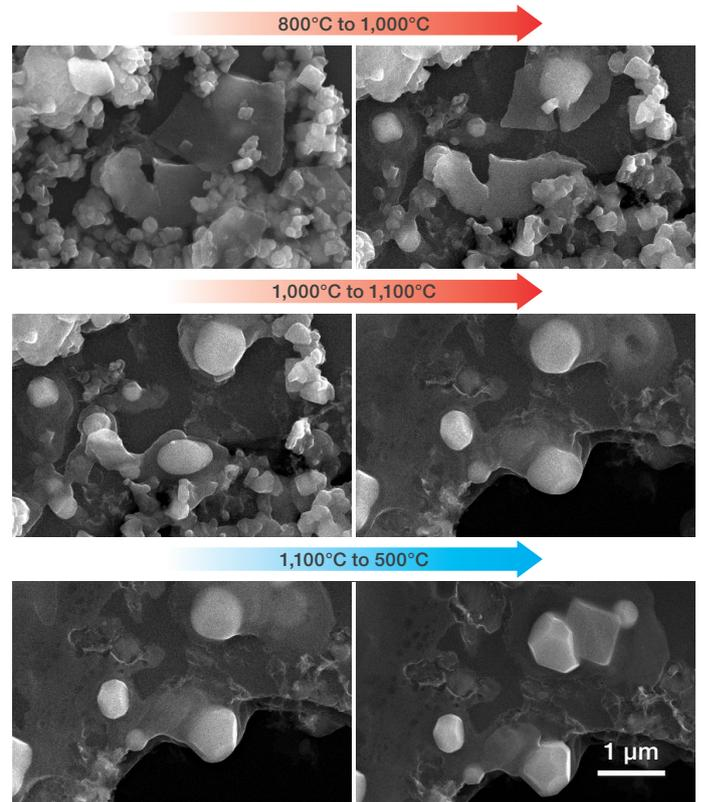
Figure 3. Microstructural changes of the area of interest during the heating and cooling processes. Acc voltage 20 keV, beam current 0.13 nA.
