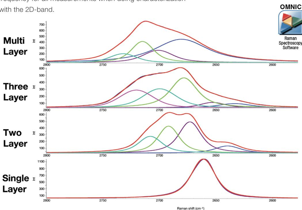
Figure 4. The 2D-band exhibits distinct band shape differences according to the number of layers present.
