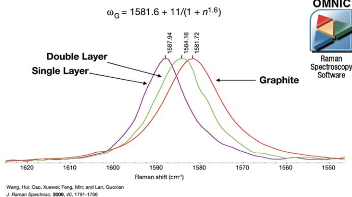
Figure 2. The G-band position is a function of layer thickness. As the number of layers increase, the band shifts to lower wavenumber, collected with 532 nm excitation.
