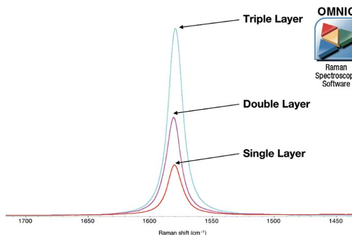
Figure 3. There is a linear increase in G-band intensity as the number of graphene layers increases, collected with 532 nm excitation.
