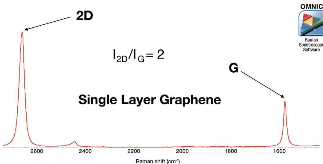
Figure 5. Single layer graphene can be identified by the intensity ratio of the 2D-band to G-band.
