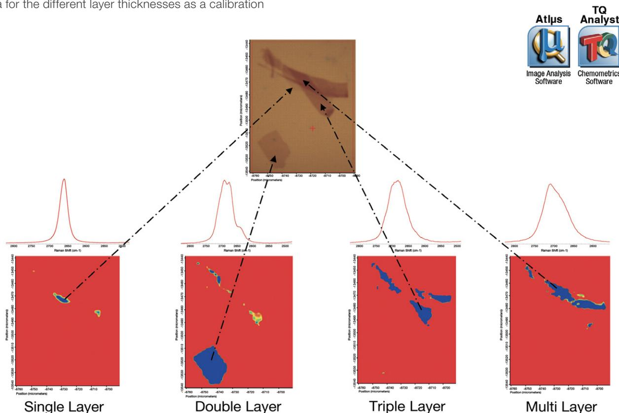
Figure 7. Discriminant analysis applied to the graphene Raman Atlas Software image shown in Figure 6. The analysis gives the distribution of the different layer thicknesses contained in the sample.
