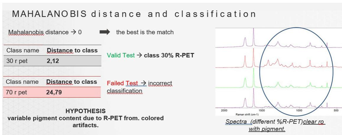
Figure 4. Examples of valid and failed classifications for R-PET samples.
