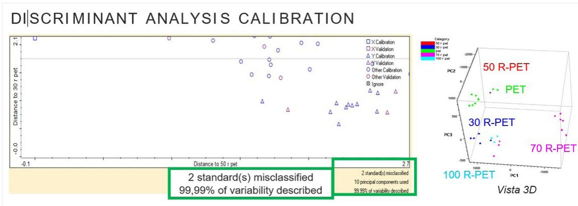
Figure 3. Discriminant analysis calibration and 3D plot of standards with different R-PET content, plotted according to the first three principal components.
