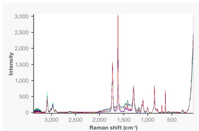
Figure 2. Raman spectra of several samples with varying ratios of virgin and recycled PET. (R-PET content ranging from 0% to 100% by weight.)
