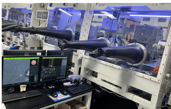
Figure 3. The Thermo Scientific Phenom Pharos Desktop SEM in the GIS.
