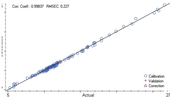
Figure 3: Calibration curve and residual for ethanol in wine.
