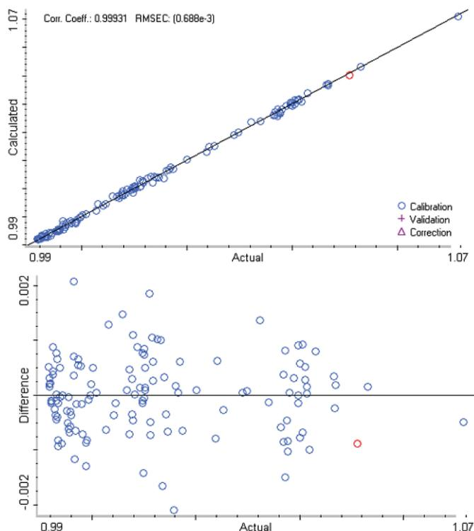
Figure 5: Calibration curve and residual for density in wine.
