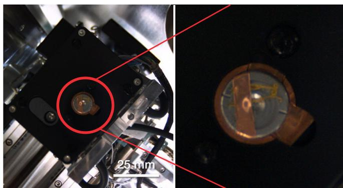
Figure 6. Navigation camera image showing the WetSTEM stage used for the top-down investigation. Two flower sepals are fixed to the Peltier stub using a small piece of copper tape.
