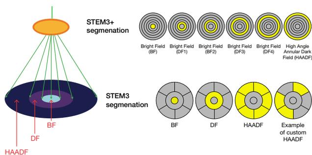
Figure 2. Schematic of the STEM3/3+ detector with two different segmentation systems.
