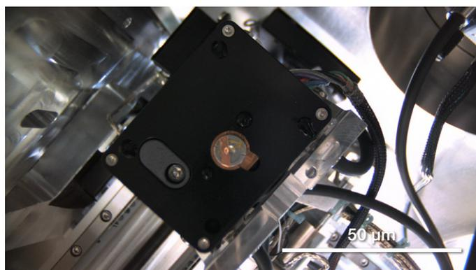
Figure 1. Navigation camera image showing the WetSTEM stage mounted in the SEM chamber.
