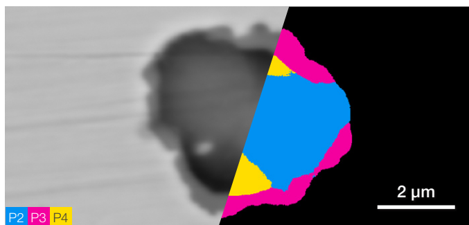
ChemiPhase image showing different phases present in a complex inclusion in steel.
