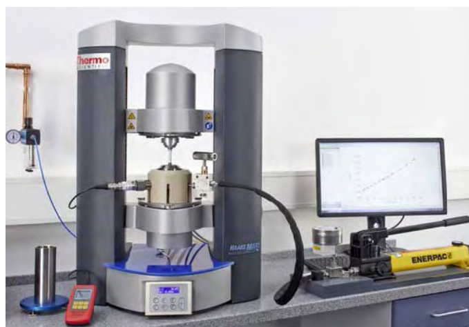
Figure 1: HAAKE MARS Rheometer with pressure cell.
