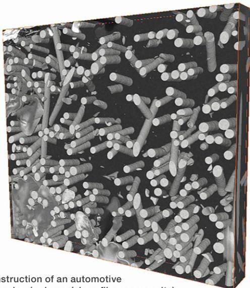
3D reconstruction of an automotive oil filter casing (polymer/glass fiber composite) acquired with a Helios Hydra CX DualBeam using O<sup>+</sup> focused ion beam and AS&V4 Software for automated serial sectioning. HFW is 350 μm.
