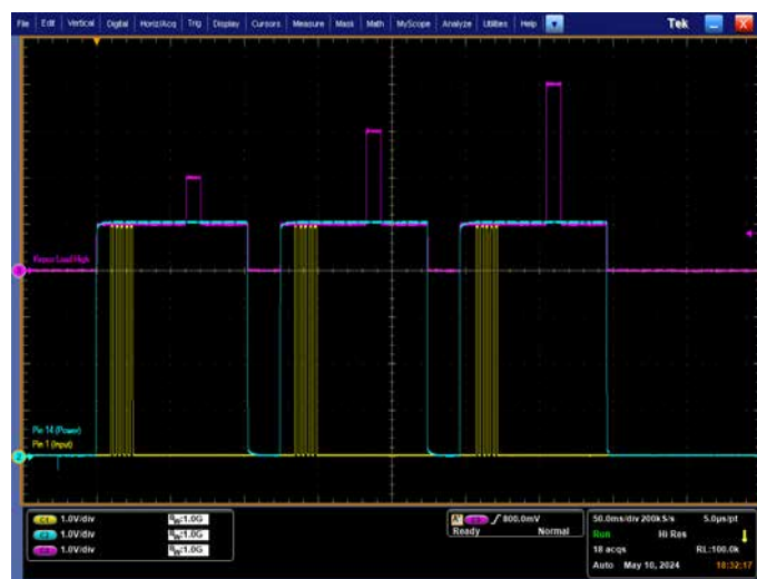
Hybrid Power Supply waveform (magenta) performing a supply over-voltage test, synchronized with internal power supply (cyan) and vectors (yellow).
