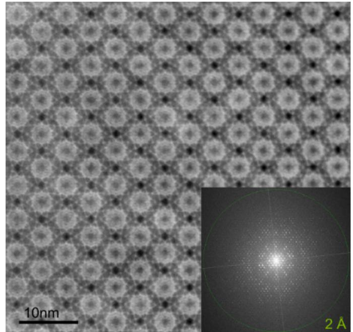
Figure 4. Metal Organic Framework (MOF) MIL-101 imaged with 0.5 pA of beam current in STEM with iDPC at 200 kV. The image is a single shot with a frame time of 23.5 seconds and the complex structure can be seen with 2 Å resolution. Specimen courtesy of Professor Y. Han, King Abdullah University of Science and Technology.
