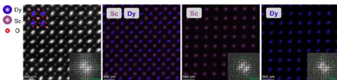
Figure 1. DyScO<sub>3</sub> specimen investigated with a Spectra 200 S/TEM. The combined ultra-high brightness of the X-CFEG, resolving power of the S-CORR and large solid angle (1.76 Sr) of the Dual-X detectors results in high signal to noise ratio, atomic resolution, raw and unfiltered EDX maps that can be collected with up to 90 pm resolution. *Sample courtesy Professor L.F. Kourkoutis, Cornell University.*
