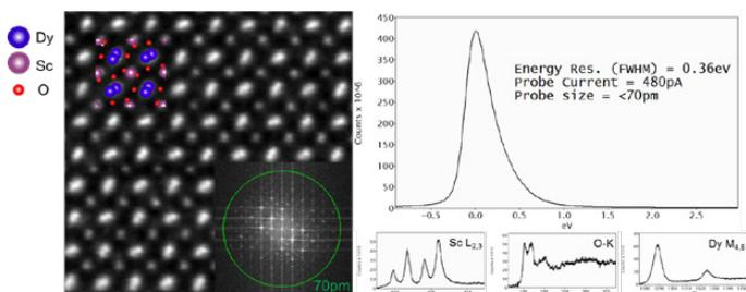
Figure 2. DyScO<sub>3</sub> specimen investigated with a Spectra 200 S/TEM. The combined ultra-high brightness of the X-CFEG, intrinsically low-energy spread of the source (<0.40 eV) and resolving power of the S-CORR results in high signal to noise ratio, Sc, O and Dy core loss edges with a sub-70 pm STEM probe. *Sample courtesy Professor L.F. Kourkoutis, Cornell University.*
