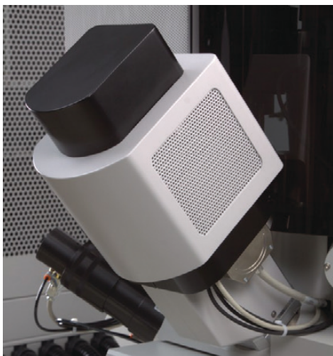
Figure 2. Thermo Scientific EasyLift Nanomanipulator
