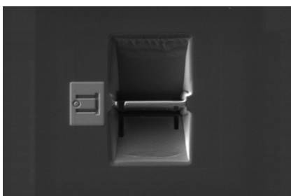
Figure 4. Sample transferred to the TEM Grid with fine precision movement
