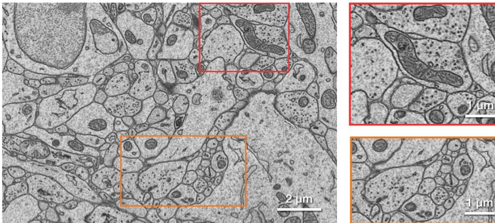
Resin-embedded, heavy-metal-stained neuronal tissue images in high vacuum using the in-lens T1 backscatter electron detector at 1.5 kV. Left image shows a low-magnification overview. Images on the right represent high-magnification images from the left image, showing contrast differences resulting from backscattered electrons.
