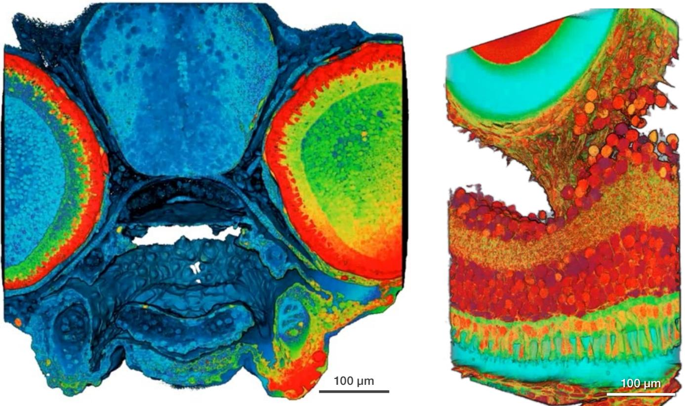
Examples of volume renderings of a zebrafish embryo head (left) and of zebrafish embryo eye tissue (right). Both samples were imaged in low-vacuum mode using the DBS detector. The zebrafish embryo head was imaged at 2 kV (100 pA) with 3 μs dwelltime. The total volume is 350 μm x 350 μm x 83 μm using a total of 829 images (with a slice thickness of 100 nm and voxel size of 42 nm x 42 nm x 100 nm). The images required 7 days of continuous imaging. Scale bar: 100 μm.
