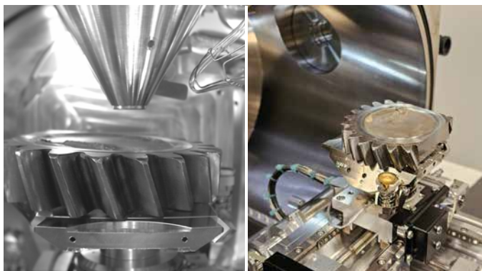
The Apreo ChemiSEM System supports a variety of industrial applications, particularly those that require characterization of large and heavy materials. It simplifies preparation by eliminating the need to cut or reduce the size of samples.
