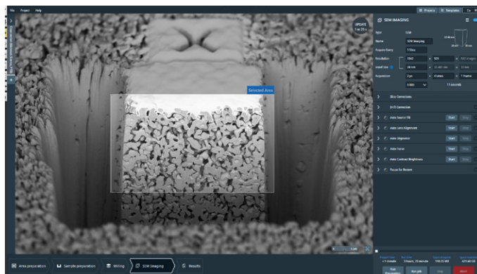
Figure 1. Auto Slice & View 5 Software’s user interface. Workflow steps are at the bottom and settings on the right. Its intuitive UI with user guidance and instructive graphics enables acquisition of high-quality 3D datasets for all users.
