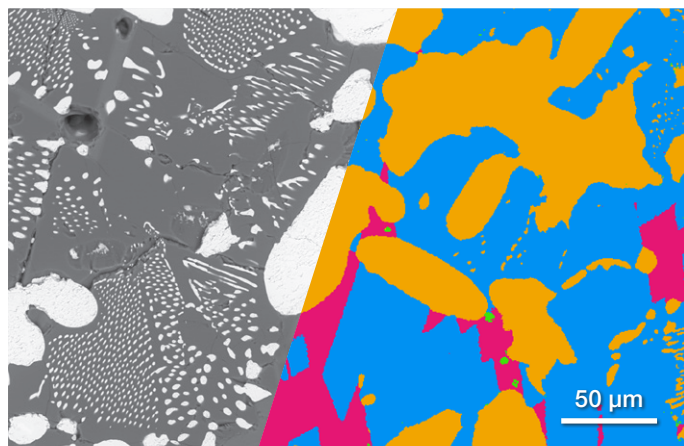
Phase analysis on a zirconia mullite polished section showing the presence of the zirconia (light orange), of the mullite phase (blue) and highlighting the presence of a third unexpected silicate phase.
