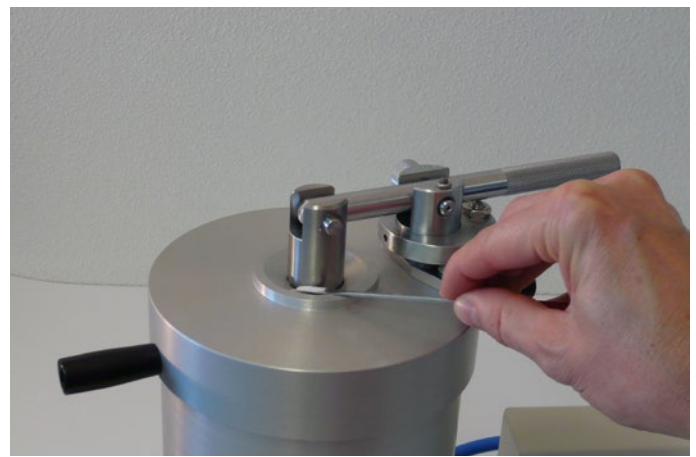
Introducing the powder in the Nebula for a proper dry dispersion
