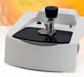
You get clean, high-quality spectra in less time across the entire mid-infrared and far-infrared<sup>†</sup> spectral range with the robust full-diamond crystal and efficient allreflective optics. Use the germanium option for difficult samples like carbon-filled polymers, or the cost-effective zinc selenide (ZnSe) option if you analyze only liquids and soft solids.
