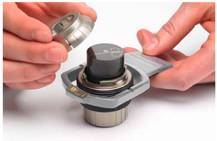
Metallurgical charge reduction sample holder
