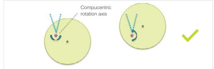
Compucentric rotation keeps the position intact.
