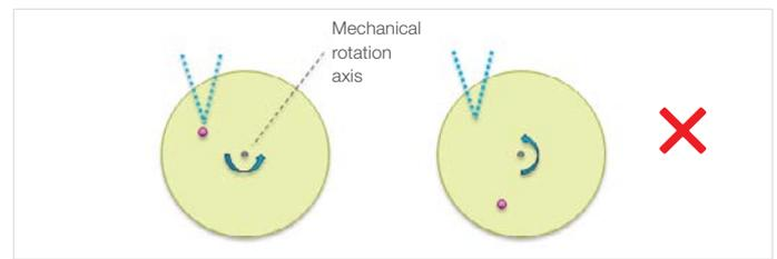
Rotating around an axis that does not coincide with the area of interest causes a shift in position. The user now has to refine the correct (x,y) position.
