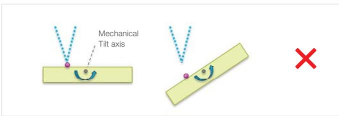
Tilting around an axis that does not coincide with the area of interest causes shifts in position and focus. The user has to make major adaptations to the SEM settings to reposition the sample and adjust the focus.
