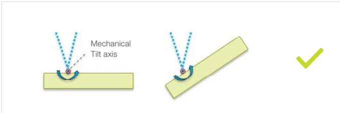
Tilting around an axis that coincides with the area of interest leaves focus and position intact.
