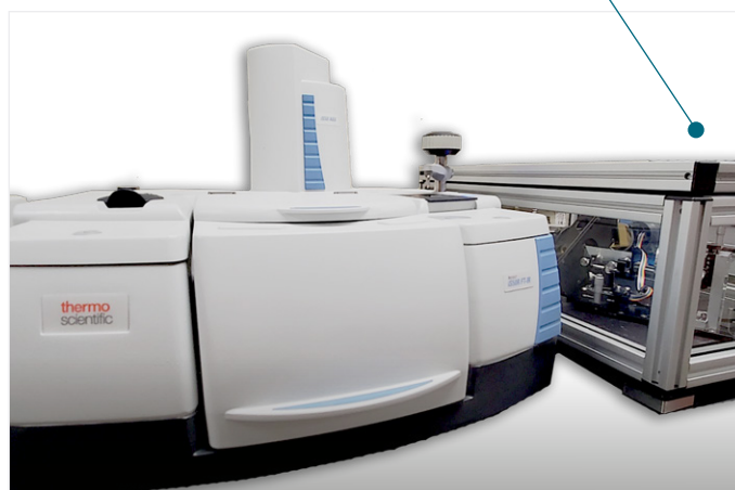
Thermo Scientific Nicolet iS50 FTIR Spectrometer with complete PM-IRRAS module.
