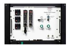
Complete dedicated solution for gas analysis. TFS Modular Gas Sampling system configured with Antaris IGS FTIR spectrometer
