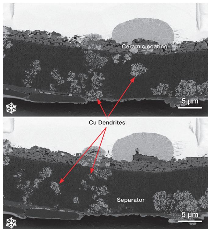
Figure 1: SEM cross section showing Cu dendrite precipitation within and penetrating the Li-ion battery separator. Sample preparation and imaging were done using the Thermo Scientific™ Scios™ 2 DualBeam™ FIB-SEM with cryo stage at  $-178^{\circ}\text{C}$ . Sample courtesy of the Sichuan New Energy Vehicle Innovation Center.
