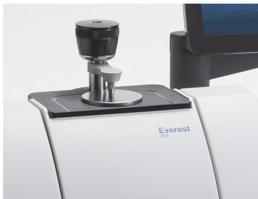
The pressure tower is designed to apply consistent pressure to the sample every time. It applies approximately 40 pounds of pressure to ensure maximal contact between the sample and the ATR crystal. Using a slip clutch mechanism, the device automatically stops applying more pressure once the maximum pressure is achieved. This protects the crystal from damage and provides consistent sampling results.
