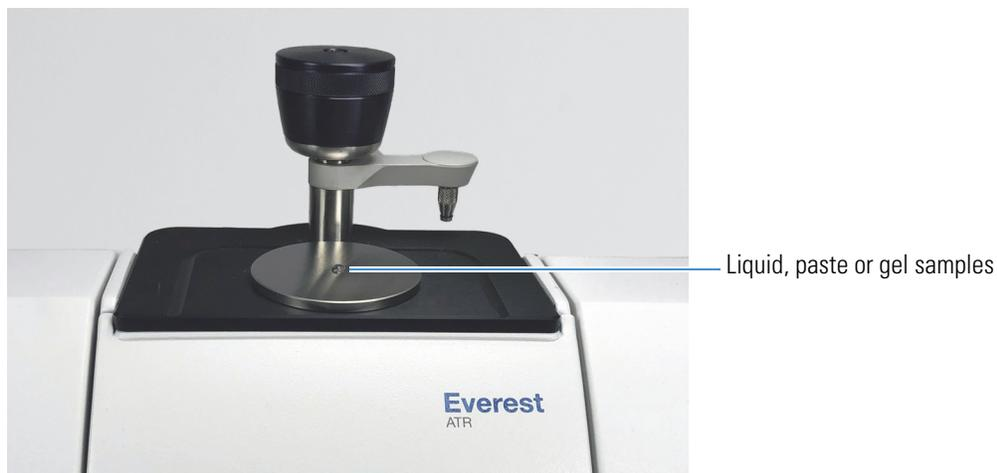
A volatiles cover is available for containing liquid samples and reducing evaporation, if needed. The volatiles cover is a flat circular plate with an O-ring on the underside. To eliminate evaporation, it can be sealed by applying pressure using the flat pressure tip.
