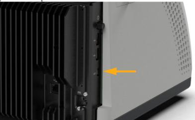
**Note** Some USB and Mini DisplayPort devices are known to interfere with the signal from wireless USB devices, such as wireless keyboards and mice. If you notice performance issues with your wireless keyboard and mouse, such as lag or delayed or missed input, use the provided USB extension cable to position the wireless USB receiver farther from the USB ports.
