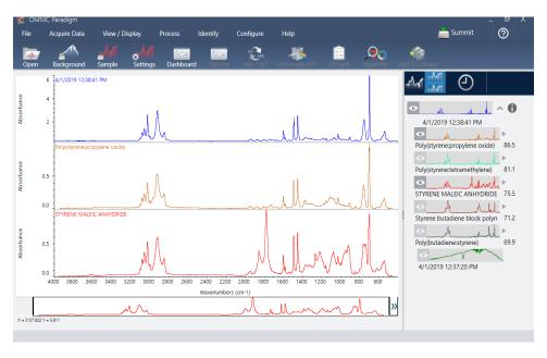
Use the spectral view to process, analyze, or explore your data in depth. Here you can process your data, find and label peaks, and optimize the view so you can more easily compare or analyze spectra.
