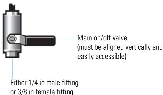
A pressure regulator is required at 20 psig. If the purge kit was purchased with the system, our service representative will install a pressure regulator and flowmeter. These components will maintain pressure and flow for optimal data collection. See the “Service” section of the user guide for more detailed information.
