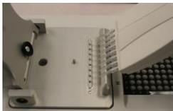
Loading samples when operating within the 8 Sample Mode.
