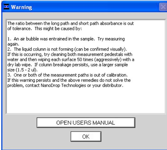
This warning occurs when a possible problem with the column is detected. The software compares the long path and short path absorbances and issues a warning to the user if the short path is not 20% of the long path absorbance, within a tolerance. The most common explanation is that the column is not forming properly due to the pedestal being “unconditioned”.
