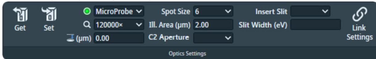
The beam diameter and magnification are used to calculate the illuminated area on the specimen.
