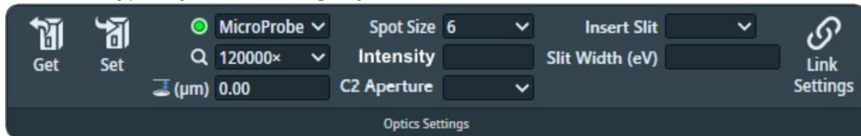
The beam diameter is displayed as an *Intensity* value. On a microscope with two condenser lenses it is not possible to calculate the beam diameter or the illuminated area on the specimen.
