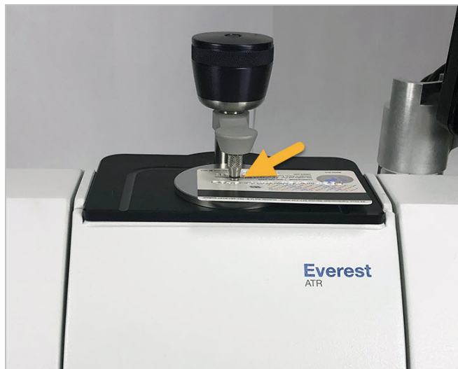
Figure 3-2: Measure a solid with ATR
