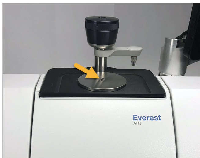
Figure 3-1: Measure a liquid with ATR
