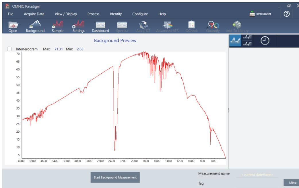
**Figure 13.** Background spectrum from a transmission accessory that has been purged
