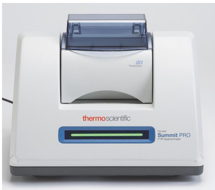
Remove any sample from your accessory or sample holder so the spectrometer can take an accurate background measurement when it's ready. The iD1 accessory cover can be open or closed. (If your transmission accessory is purged with dry air or nitrogen, keep the cover closed unless you are adding or removing a sample.)
