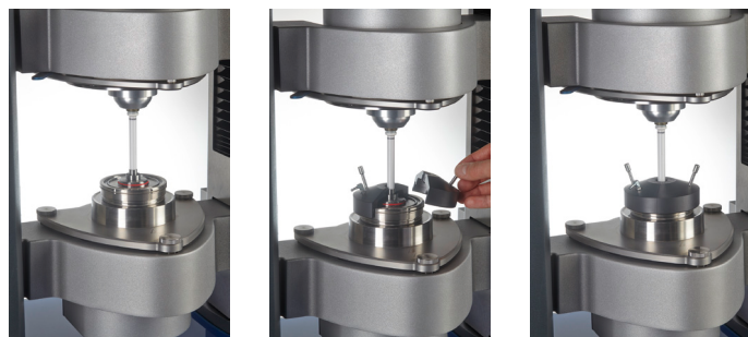
Figure 4: Parallel plate geometry in measurement position without and with sample cover.
