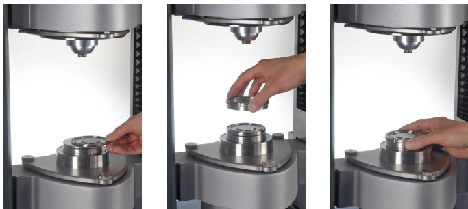
Figure 1: Mounting of a lower plate on top of a temperature module.
