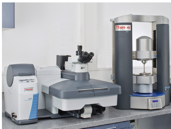
Figure 1: Combination of a HAAKE MARS rheometer with RheoRaman module and adapted Nicolet DXR Raman microscope.
